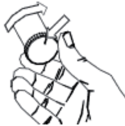
Figure 8 Coalescing Filter Maintenance 4
