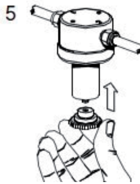
Figure 2 Particulate Filter Maintenance 2
