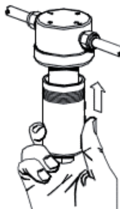
Figure 4 Particulate Filter Maintenance 4
